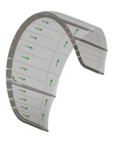
When engineering the load control paneling, we make sure that fabrics panels are warp/weft oriented, meaning that the load path runs through the yarns. Fabric and seams are then in the best position to receive tensions and maintain the original kite and wing shape.
